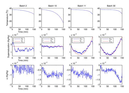
Figure 3.3: Case 1 ILC: temperature reference  $T^r$ , supersaturation S, and correction vector  $\alpha$  for the batches 2, 10, 11, and 30.
