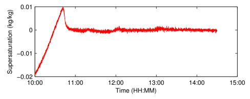
(c) The supersaturation S reaches a maximum at around 10:45 and drops to 0 afterwards.
