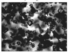
(e) t=11:19,  $T=37.29~^{\circ}\mathrm{C},~C_{\mathrm{solid}}=3\%.$  The crystals keep on increasing in number and in size. The image get darker and it becomes more and more difficult to distinguish individual crystals.
