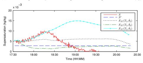
(b) The supersaturation  $S_2$  reaches a maximum of  $0.1~{\rm kg/kg}$  at 18:20 and decreases afterwards. The tracking performance is similar to the one of B2B experiment 1. None of the supersaturation models can describe the actual supersaturation dynamics with reasonable accuracy.
