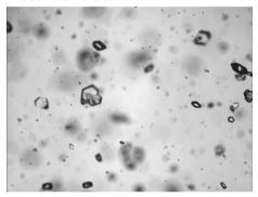
(c) t=10:45,  $T=41.3\,^{\circ}\mathrm{C},\ C_{\mathrm{solid}}=0.8\%.$  The crystals grow and increase in number due to nucleation. Most of the crystals are still individually distinguishable.
