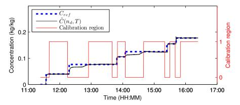
(c) Reference concentration  $C_{\text{ref}}$  (blue), concentration model  $\tilde{C}(n_D,T)$  (black) and clear solution indicator function (red).
