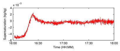
(c) The supersaturation  ${\cal S}$  reaches a maximum soon after the seeding and drops to 0 afterwards.
