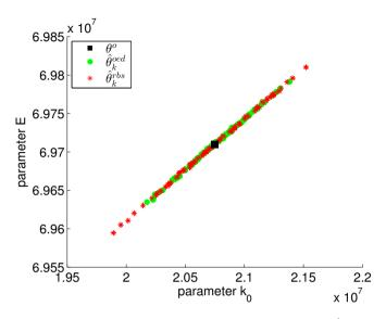
Figure 5.5: Scatter plot for the first two coordinates of  $\theta_o$ ,  $\hat{\theta}_k^{\text{oed}}$  and  $\hat{\theta}_k^{\text{rbs}}$ .
