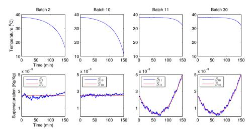
Figure 3.4: Case 1 IIC: temperature reference  $T^r$  and supersaturation S for the batches 2, 10, 11, and 30.
