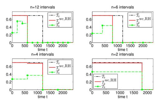
Figure 4.4: Total cost  $\mathcal{T}_k^e$ , worst-case total cost  $\mathcal{T}_k^{\mathrm{wc,RH}}$ , and constraint  $\bar{\mathcal{T}}_k$  vs. time t in Case 1 (n=12), Case 2 (n=6), Case 3 (n=4) and Case 4 (n=2) intervals. The green circles denote the time instants corresponding to the start of a learning interval.
