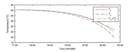
(a) Reference temperature  $T_2^r$ , measured temperature  $T_2$  and temperature model  $F_{TT^r}(T_2^r)$ .
