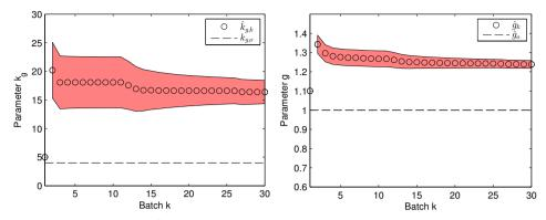
(a) Estimated parameter  $\hat{k}_g$  vs batch number. (b) Estimated parameter  $\hat{g}$  vs batch number.
