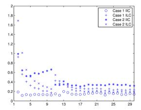
Figure 3.9: RMSE of the supersaturation vs. batch number for IIL and ILC in Case 1 and 2.
