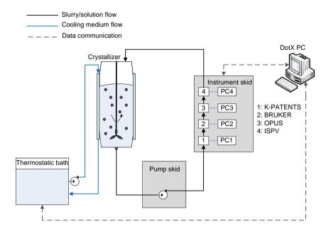
Figure 6.1: A schematic representation of the experimental setup.
