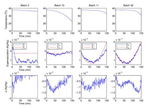
Figure 3.6: Case 2 ILC: temperature reference  $T^r$ , supersaturation S, and correction vector  $\alpha$  for the batches 2, 10, 11, and 30.
