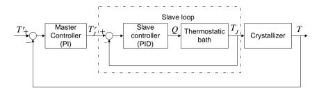
Figure 6.7: The master-slave control scheme for the temperature of the crystallizer.
