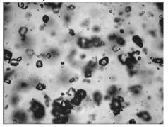
(d) t=10:52,  $T=40.64~^{\circ}\mathrm{C},~C_{\mathrm{solid}}=1.4\%$ . More and more crystals are present. Some of the crystal start to overlap on each other on the image.
