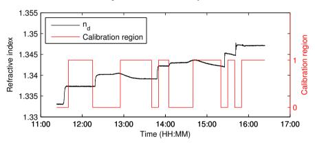
(b) Refractive index  $n_d$  from the K-Patents (black) and clear solution indicator function (red).
