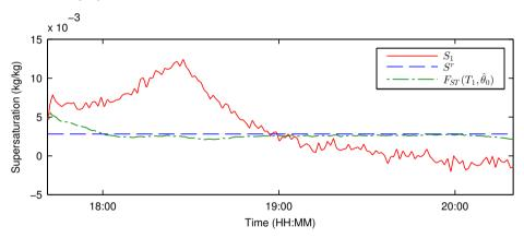
(b) The supersaturation  $S_1$  reaches a maximum value of  $0.012 \,\mathrm{kg/kg}$  at 18:30 and decreases afterwards. The trajectory is rather far from the set-point  $S^r$ .
