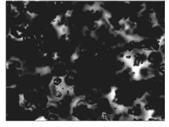
(f) t=12:05,  $T=32.10~{\rm ^{\circ}C},~C_{\rm solid}=5.3\%$ . The solid content is very high and the image is almost completely dark. single crystals are hardly distinguishable even for a human eye.
