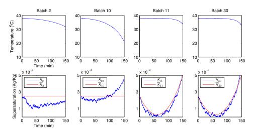
Figure 3.7: Case 2 IIC: temperature reference  $T^r$  and supersaturation S for the batches 2, 10, 11, and 30.
