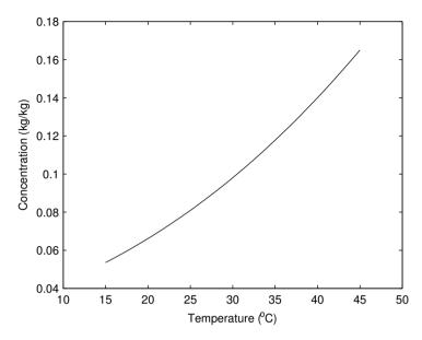
Figure 6.9: The solubility line of Succinic acid in water estimated from laboratory analysis by DSM.
