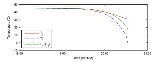
(a) Reference temperature  $T_3$ , measured temperature  $T_3$  and temperature model  $F_{TT^r}(T_3^r)$ .
