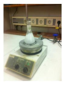
Figure 6.19: The second flask is stirred for 10 minutes with a magnetic stirrer. A well-dispersed seed suspension is obtained.
