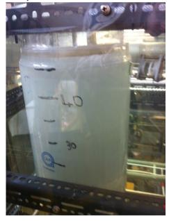
(d) During the cooling down, the solid content in the crystallizer increases and the slurry gets more and more turbid.
