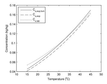
Figure 6.18: Experimental solubility with Fumaric acid  $C_{\rm s,exp,fum}(T)$ , experimental solubility based on the pure system  $C_{\rm s,exp}(T)$  and solubility from laboratory analysis  $C_{\rm s,lab}(T)$ .
