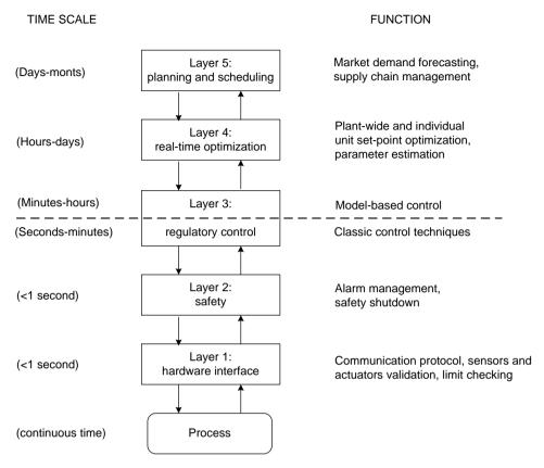
Figure 1.1: The five-layer architecture of modern process control software. Adapted from Nof (2009).
