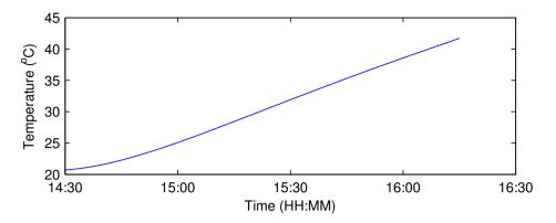
(a) Measured temperature inside the crystallizer.
