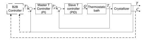
Figure 6.23: The control architecture for batch to batch control.
