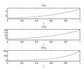
Figure A.1: Optimal input  $u^o(t)$ , state  $x^o(t)$ , and energy  $E^o(t)$  obtained using the PMP principle and solving the associated BVP analytically.
