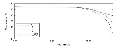
(a) Reference temperature  $\mathcal{T}_4^r$  and measured temperature  $\mathcal{T}_4$  inside the crystallizer.
