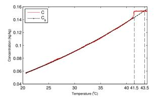
Figure 6.14: C-T plane of the unseeded batch crystallization experiment. The Metastable Zone Width is approximately 2  $^{\circ}$ C.
