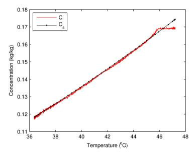
Figure 6.17: C-T plane of the first seeded crystallization experiment.
