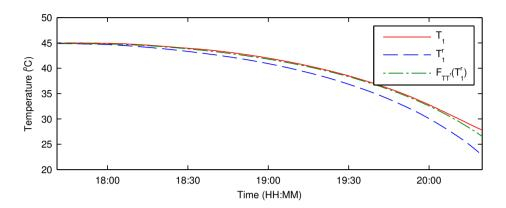
(a) Reference temperature  $T_1^r$ , measured crystallizer temperature  $T_1$  and temperature model  $F_{TT^r}(T_1^r)$ . The measured crystallizer temperature  $T_1$  is close to the temperature model  $F_{TT^r}(T_1^r)$ , as desired.
