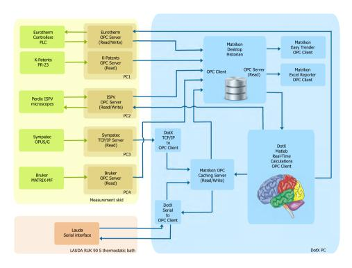
Figure 6.5: Software architecture of the experimental setup.
