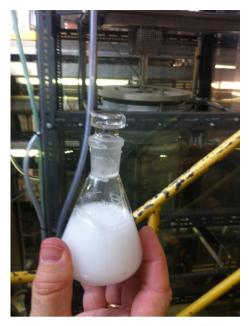
(a) The temperature in the crystallizer is  $45\ ^{\circ}\mathrm{C}$  and the solution is clear.
