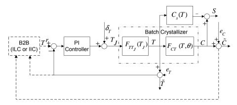
Figure 3.1: The overall B2B+PI control scheme.
