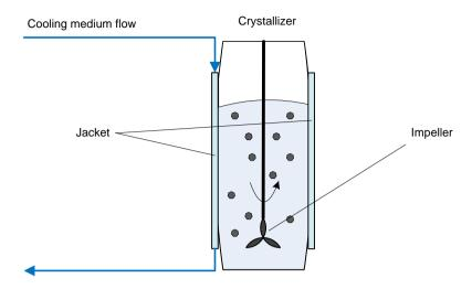
Figure 2.2: Schematic representation of a batch cooling crystallizer. The crystallizer temperature is manipulated by circulating a fluid medium in *jacket*. The content of the crystallizer is mixed with the help of an impeller.
