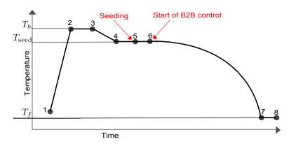
Figure 6.24: The steps of the experimental procedure for the B2B experiments. The B2B algorithm is used to determine the cooling trajectory at the step 6 of the procedure.
