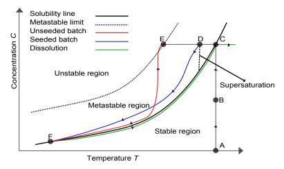
Figure 2.1: The phase diagram of the ideal experiment.
