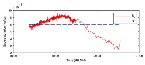
(b) The supersaturation  $S_3$  is relatively close to the set-point  $S^r$  for the first part of experiment.
