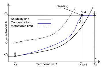
Figure 2.3: Steps of a batch cooling crystallization.
