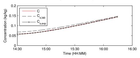
(b) Solubility from laboratory analysis  $C_{s,lab}(T)$ , measured concentration C, and experimental solubility  $C_{s,exp}(T)$ .
