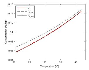
Figure 6.12: C-T plane of the heatup experiment for the determination of the solubility. The solubility  $C_{\rm s,exp}$  is interpolated based on the measured concentration and temperature data. There is a mismatch between  $C_{\rm s,exp}$  and the solubility obtained from laboratory data  $C_{\rm s,lab}$ .
