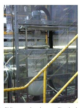
Figure 6.2: The 50-liters vessel used as crystallizer for the experiments.
